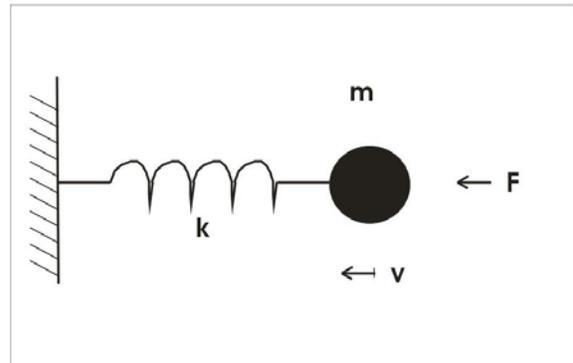
Figure 1. Basic Mass-Spring Vibrator model
