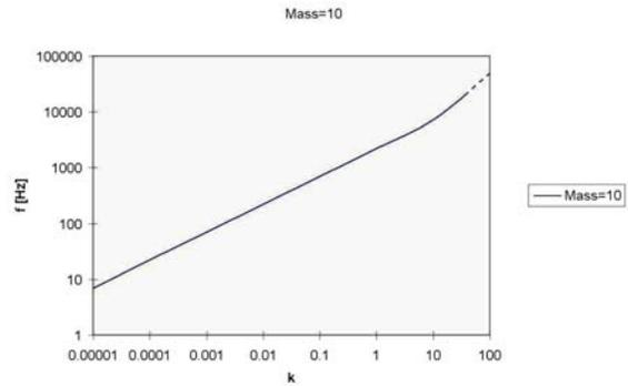
**Figure 3.** Linearity of difference equation calculation as the spring constant  $k$  and frequency  $f$  increase (sample frequency=44.1kHz)
